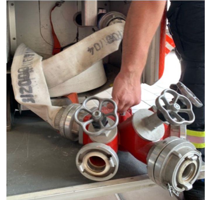
Hose on the distributor
